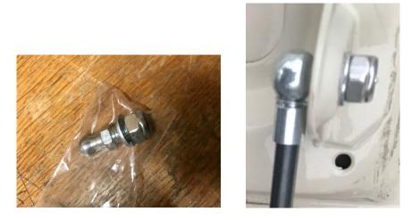
Take the strut and remove the two securing pins from each end of the strut.
