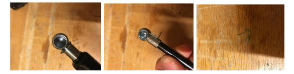
Frist place the thicker end of the strut over the lower ball bolt, they are a tight fit, so it may need a tap to drive it home. You will hear it pop on. Now lift the lid and pop the skinny end of the strut on the top ball bolt.
